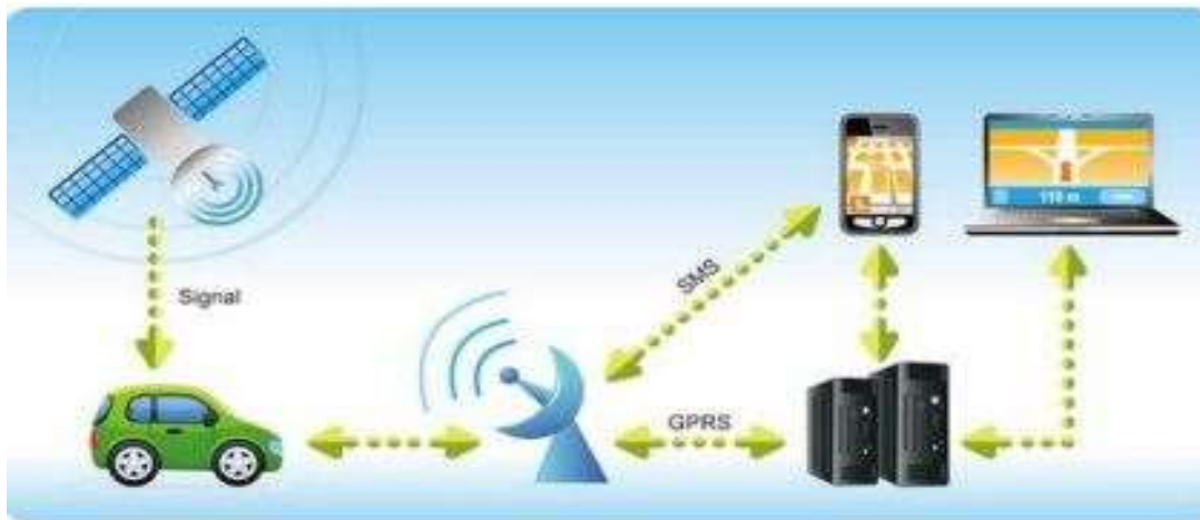
Figure 1: Car tracking system using GPS and GSM
